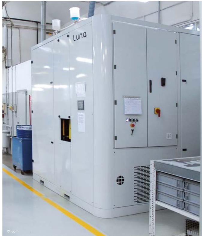
The L.UN.A. 2 cleaning system was installed within a small space in the machining department.
